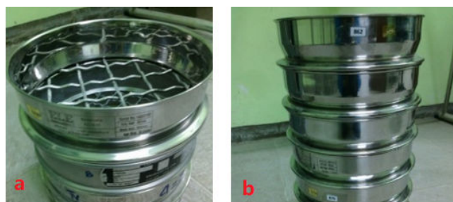
Fig. 1. (a) Coarse Aggregate Sieve ; (b) Fine Aggregate Sieve
