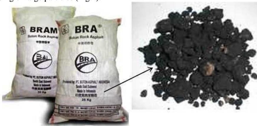
Fig. 1. Buton Bitumen Nusantara in sacks on the left side and BNRA in large particles on the right side
