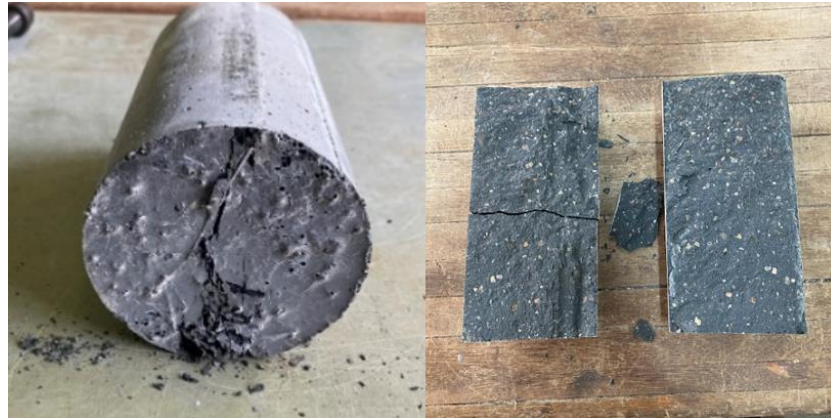
Fig. 7. Failure pattern after splitting tensile test of PFRSCHPC (left) and SCHPC (right)
