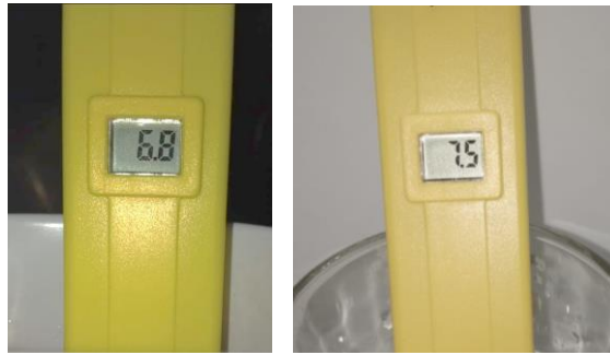
Figure 1. The degree of acidity (pH) of mineral water used to immerse magnetic dental attachments
